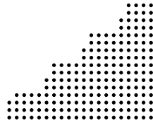
Figure 3: Bit heap obtained for a 16-bit, 8-tap half-sine pulse shaping FIR filter operator FixHalfSine
