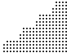
Figure 10: Bit heap obtained for a 16-bit, 8-tap half-sine pulse shaping FIR filter operator FixHalfSine
